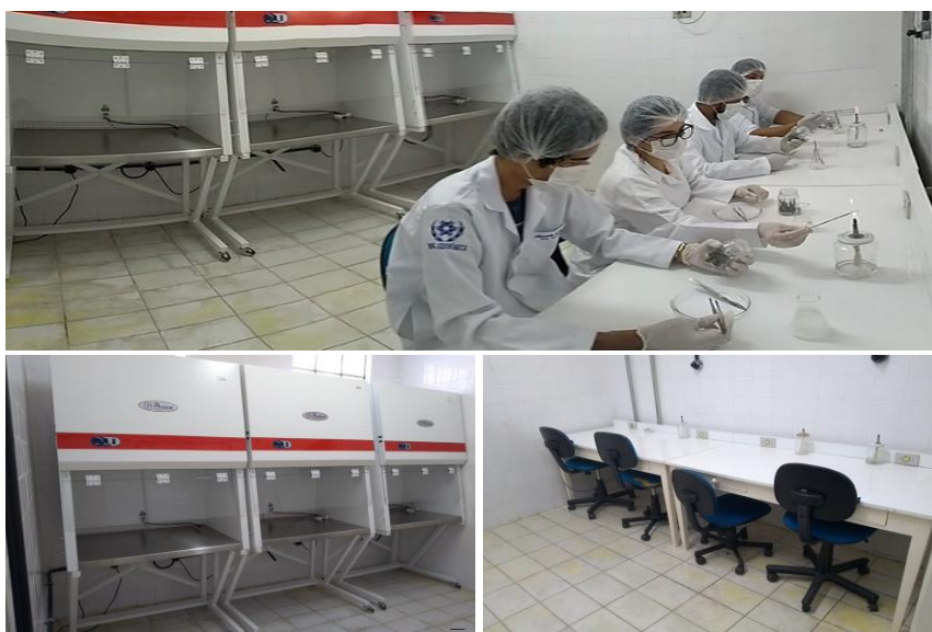
Figure 1: Environment where experiments were carried out to check the feasibility of aseptic handling of cultures outside the laminar flow hood. A: Overview of the inoculation room, with operators working outside the laminar flow hoods; B: Laminar flow hoods used as environment filters; C: Benches on which flasks were handled (Pictures: Juliana Martins Ribeiro).
