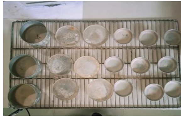
Figure 1. Results of soil texture analysis using the pipette method.
